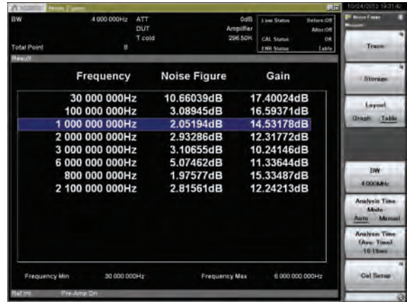
Measurement Result: Example of List display (Frequency Mode: List, Screen Layout: List)
